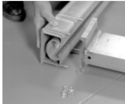
5. Mount the lower frame weldment (Ref.#6) to the winch post extrusion (Ref.#14) using two (2) 3/8" X 5-3/16" X 3-7/8" square u-bolts (Ref.#30) as shown. Secure with 3/8" flange lock nuts.
