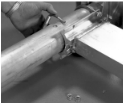
7. Also mount the guide post tube to the opposite end of the lower frame tube using two (2) 3/8" X 3-7/8" X 3-7/8" SUB's. Secure with 3/8" flange lock nuts.
