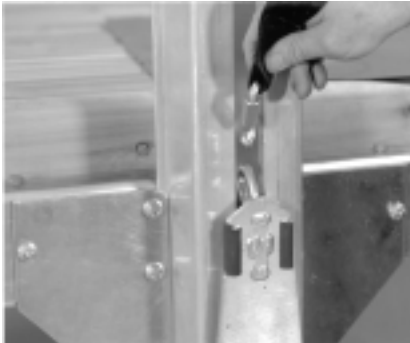
13. Connect the end of the winch strap to the platform weldment assembly as shown.
