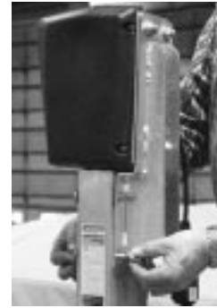
12. Mount the electric winch assembly that is attached to the mounting plate to the winch post using four (4) 3/8" X 3-3/4" hex bolts. Slide the electric control holder over the end of the one of the lower 3/8" X 3-3/4" hex bolts on either side of the electric winch. See diagram on page 2. Secure with four (4) 3/8" flange lock nuts. Place the electric controller unit into the electric control holder.
