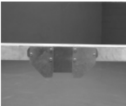
16. Mount the hoist attach plate (Ref.#11) to the winch post mounting plate over the six (6) 3/8" X 1-1/2" carriage bolts as shown. Secure with 3/8" flange lock nuts.
