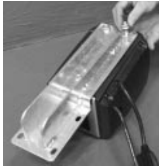
11. Mount the electric winch to the winch mounting plate using two (2) 1/2" X 1" hex bolts in the top two (2) mounting holes and one (1) 3/8" X 1" hex bolt in the single lower mounting hole. Secure with two (2) 1/2" lock washers and two (2) 1/2" hex nuts. Secure the 3/8" X 1" hex bolt with a 3/8" lock washer and a 3/8" hex nut.
