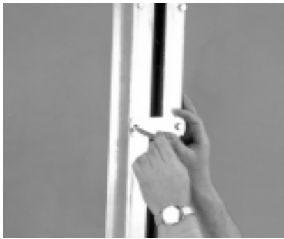
14. Mount the stop plate (Ref.#12) to the winch post extrusion using two (2) 3/8" X 3-3/4" hex bolts (Ref.#22). Secure with 3/8" flange lock nuts.
