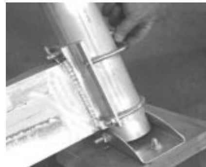
6. Also mount the guide post tube to the opposite end of the lower frame tube using two (2) 3/8" X 3-7/8" X 3-7/8" RUB's. Secure with 3/8" flange lock nuts.
