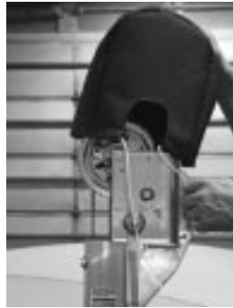
20. Slide the blue cover over the winch assembly as shown. This cover is used to protect the winch assembly from the weather.
