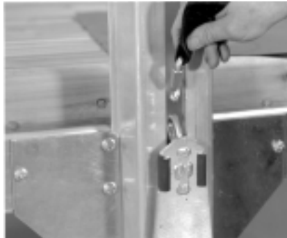
14. Unwind the strap from the winch. Connect the end of the winch strap to the platform weldment assembly as shown.
