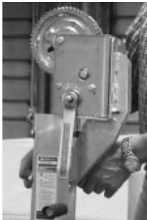
13. Mount the winch assembly with winch mounting bracket to the winch post extrusion using the four (4) 3/8" X 3-3/4" hex bolts just installed. Place a 3/8" flat washer on each of the four (4) 3/8" X 3-3/4" hex bolts. Insert them into the holes provided in the top of the winch post extrusion. Secure with 3/8" flange lock nuts.
