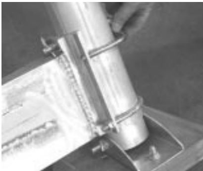
7. Also mount the guide post tube to the opposite end of the lower frame tube using two (2) 3/8" X 3-7/8" X 3-7/8" RUB's. Secure with 3/8" flange lock nuts.
