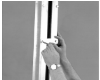
15. Mount the stop plate to the winch post extrusion using two (2) 3/8" X 3-3/4" hex bolts. Secure with 3/8" flange lock nuts.
