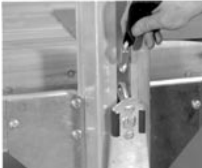
13. Connect the end of the winch strap to the platform weldment assembly as shown. NOTE: The strap must be free of any twisting.
