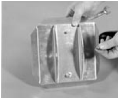
2. Install the aluminum base pad channel clamp to the base pad using two (2) 3/8" X 1" hex bolts and two (2) 3/8" flange lock nuts.
