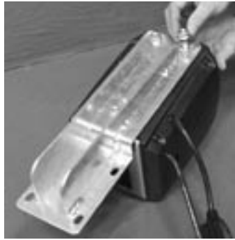
11. Mount the electric winch to the winch mounting plate using two (2) 1/2" X 1" hex bolts in the top two (2) mounting holes and one (1) 3/8" X 1" hex bolt in the single lower mounting hole. Secure with two (2) 1/2" lock washers and two (2) 1/2" hex nuts. Secure the 3/8" X 1" hex bolt with a 3/8" lock washer and a 3/8" hex nut.
