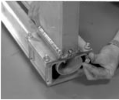
10. Secure the cable end to the under side of the lower frame weldment with a 3/8" flat washer and 3/8" hex nut.
