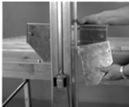
17. Mount one (1) hoist attach plate to the winch post mounting channel using three (3) 3/8" X 1" carriage bolts. Secure with 3/8" flange lock nuts. NOTE: The hoist attach plate must be hooked over the lip on the winch post extrusion. Place the other hoist attach plate onto the opposite side of the winch post extrusion - be sure this plate extends over the lip of the winch post extrusion before tightening.
