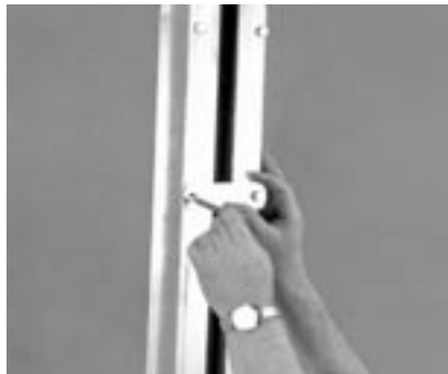
14. Mount the stop plate to the winch post extrusion using two (2) 3/8" X 3-3/4" hex bolts. Secure with 3/8" flange lock nuts.
