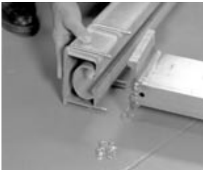
4. Mount the lower frame weldment to the winch post extrusion using two (2) 3/8" X 5-3/16" X 3-7/8" square u-bolts as shown. Secure with 3/8" flange lock nuts.
