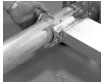
6. Also mount the guide post tube to the opposite end of the lower frame tube using two (2) 3/8" X 3-7/8" X 3-7/8" SUB's. Secure with 3/8" flange lock nuts.
