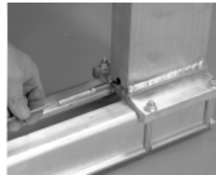
9. Run the threaded end of the cable through the lower frame weldment as shown.
