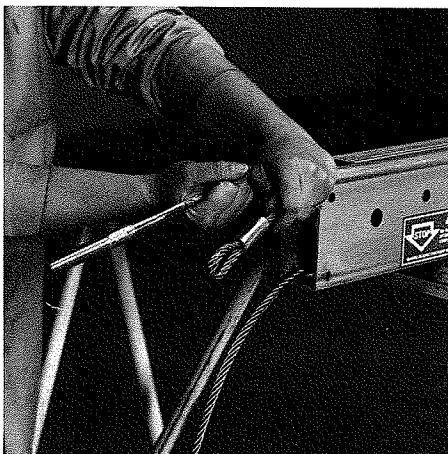
10C. Hold threaded end cable and cable with loop, as sheave assembly is being pulled through winch tube with the cable threading handle.
