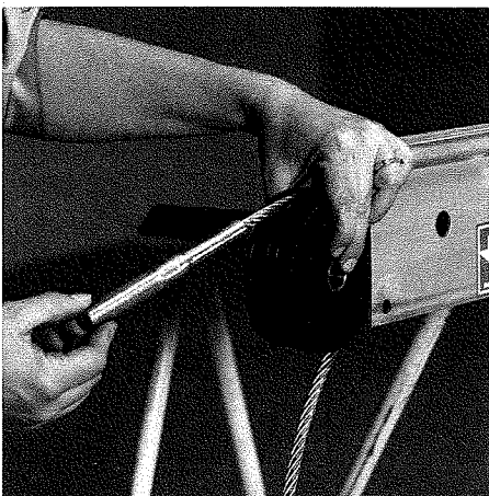
15. Install the double sheave assembly in the winch end of the winch tube with the lift cable (cable with threaded end) over the top of the left pulley and the winch cable under the pulley on the right.
