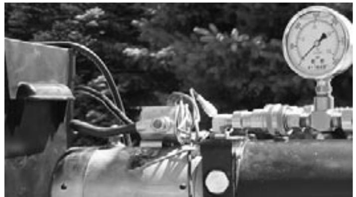
The pressure gauge is used to determine whether the output pressure of the hydraulic pump was properly adjusted when it was assembled. (Proper setting is 2450 PSI.)
